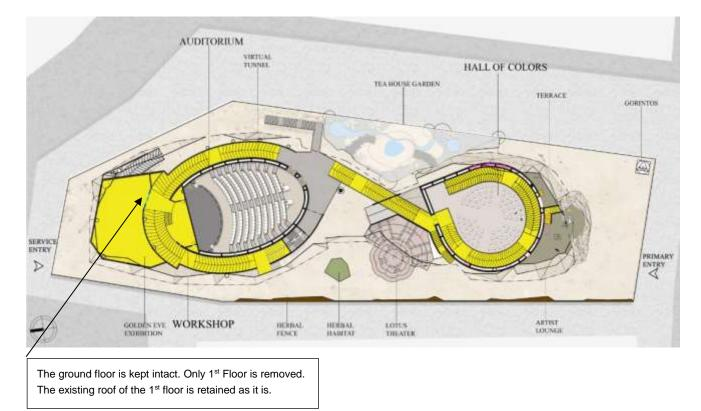
The removed portion are shown in yellow color in the schematic drawing below.
